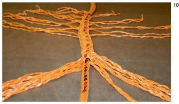
The splice is turned around and it is now possible to start on splicing area two with splicing end 2.
