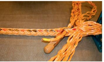
Take the spike under the first two strands and pull the first set of four strands over one red and under two black.
