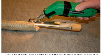
Use a heat knife and a spike to cut the protective jacket and peel it back from the splicing areas and splicing ends.
