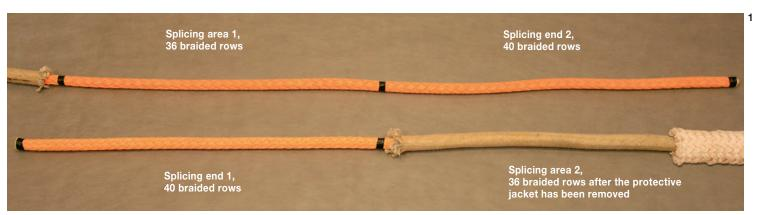
Before starting the splice, it is important that the ends to be spliced are not twisted and are tension-free before they are brought together.
