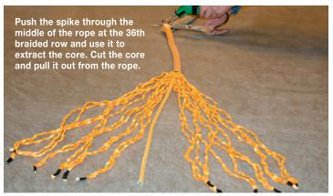
Unbraid the splicing end into twelve two-strands and tape the ends of each pair together.
